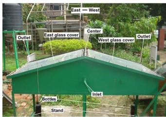
Figure 1: A photograph of double slope solar still.
